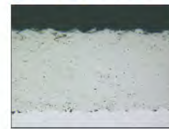
Cross-section metallograph of WC-10Ni coating
