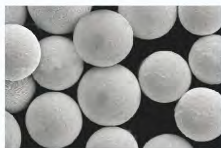
SEM morphology of spherical cast tungsten carbide
