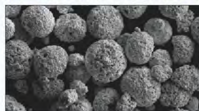
Typical cross-section and surface morphology of WC-12Co thermal spray powder
