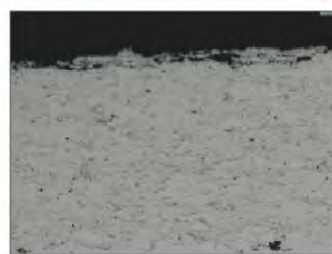
Cross-section metallograph of Cr 3 C 2 -25NiCr coating
