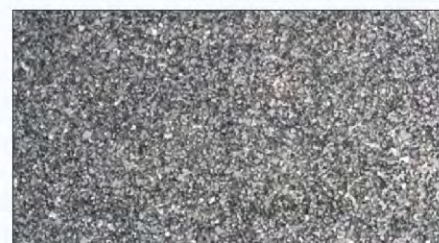
Microstructure of cemented carbide pellet X1000
