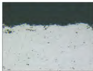
Cross-section metallograph of WC-12Ni coating
