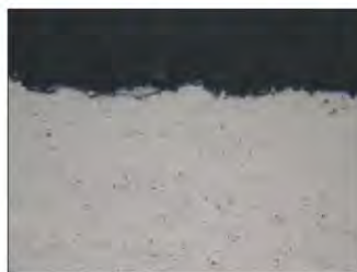
Cross-section metallograph of WC-12Co coating
