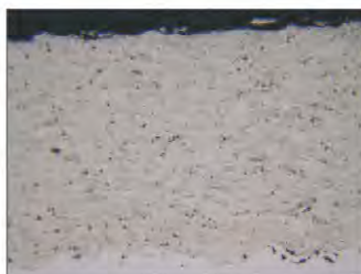
Cross-section metallograph of Cr 3 C 2 -37WC-18NiCoCr coating
