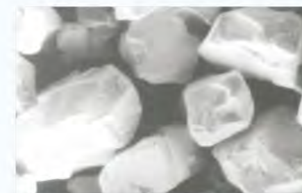
SEM morphology of macrocrystallite tungsten carbide
