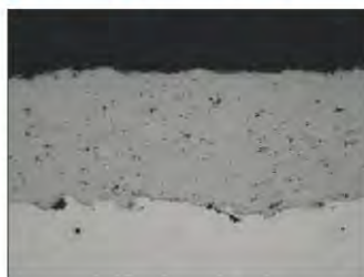
Cross-section metallograph of WC-15NiCr coating
