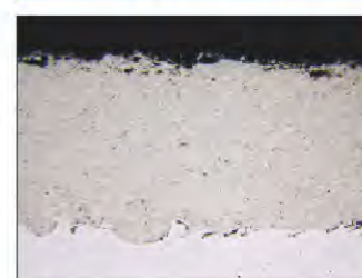
Cross-section metallograph of WC-20Cr-7Ni coating
